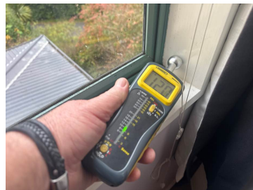
Very high moisture reading in this area bunk room
