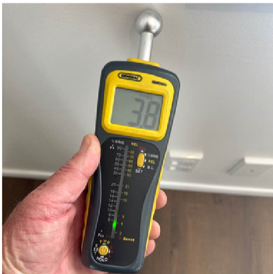
Low moisture reading, green = Good
