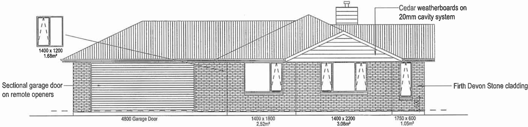
EAST ELEVATION Window Area: 8.33m²
