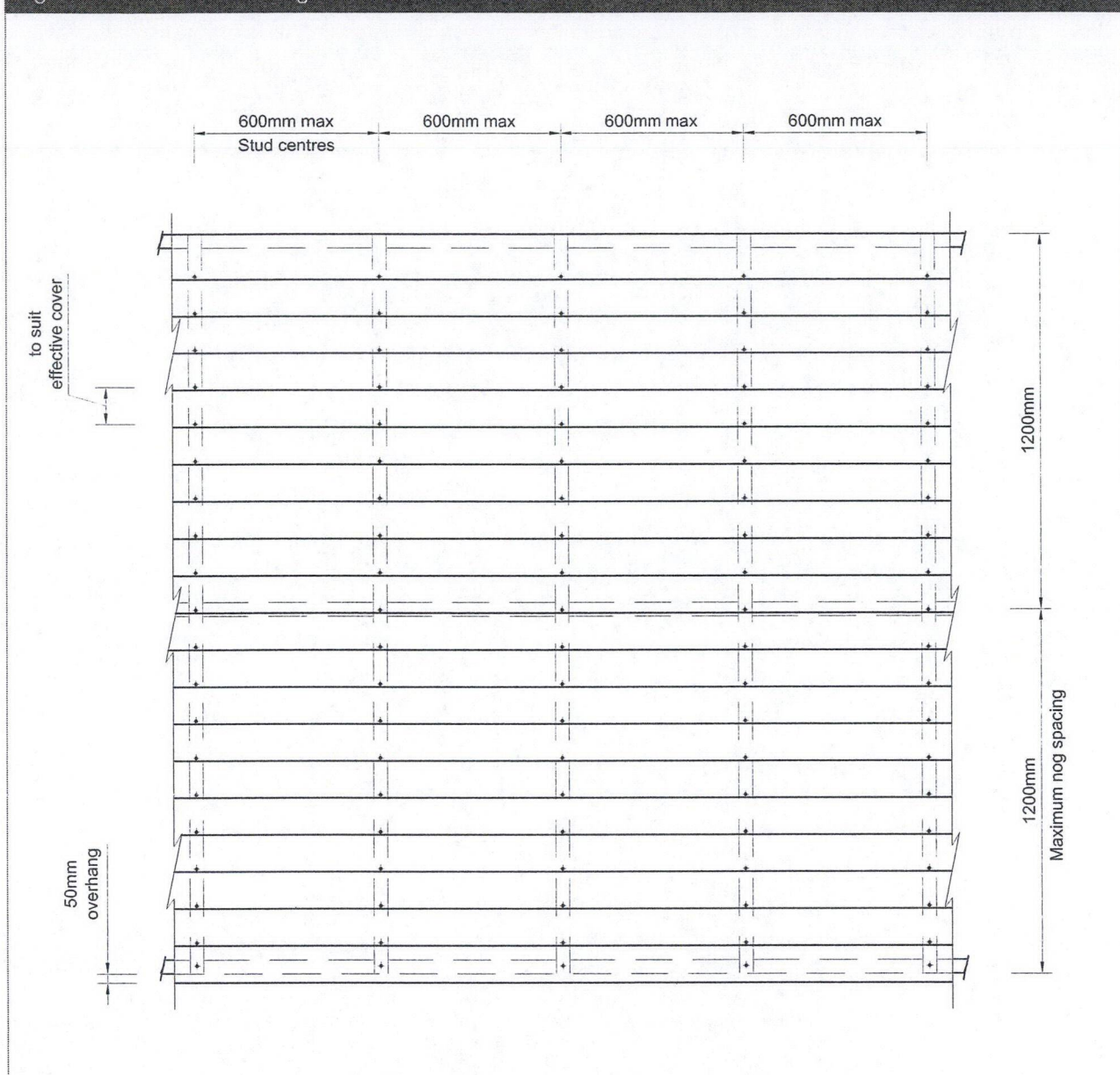
Figure 2: Direct fix sheet fixing setout
