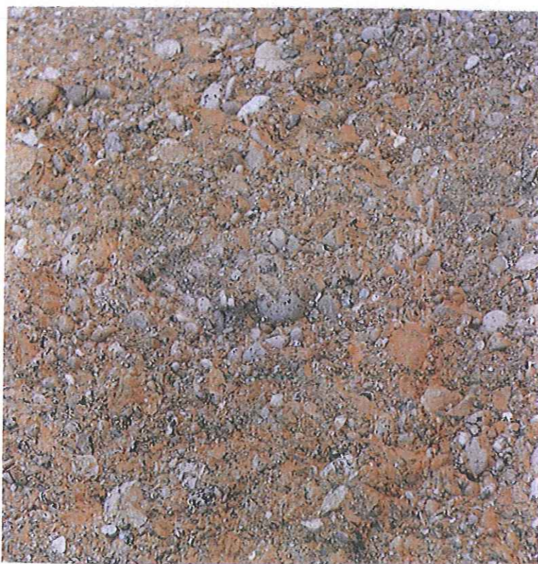
Typical less weathered Moutere Gravel exposure in cut batter opposite Lot 7
