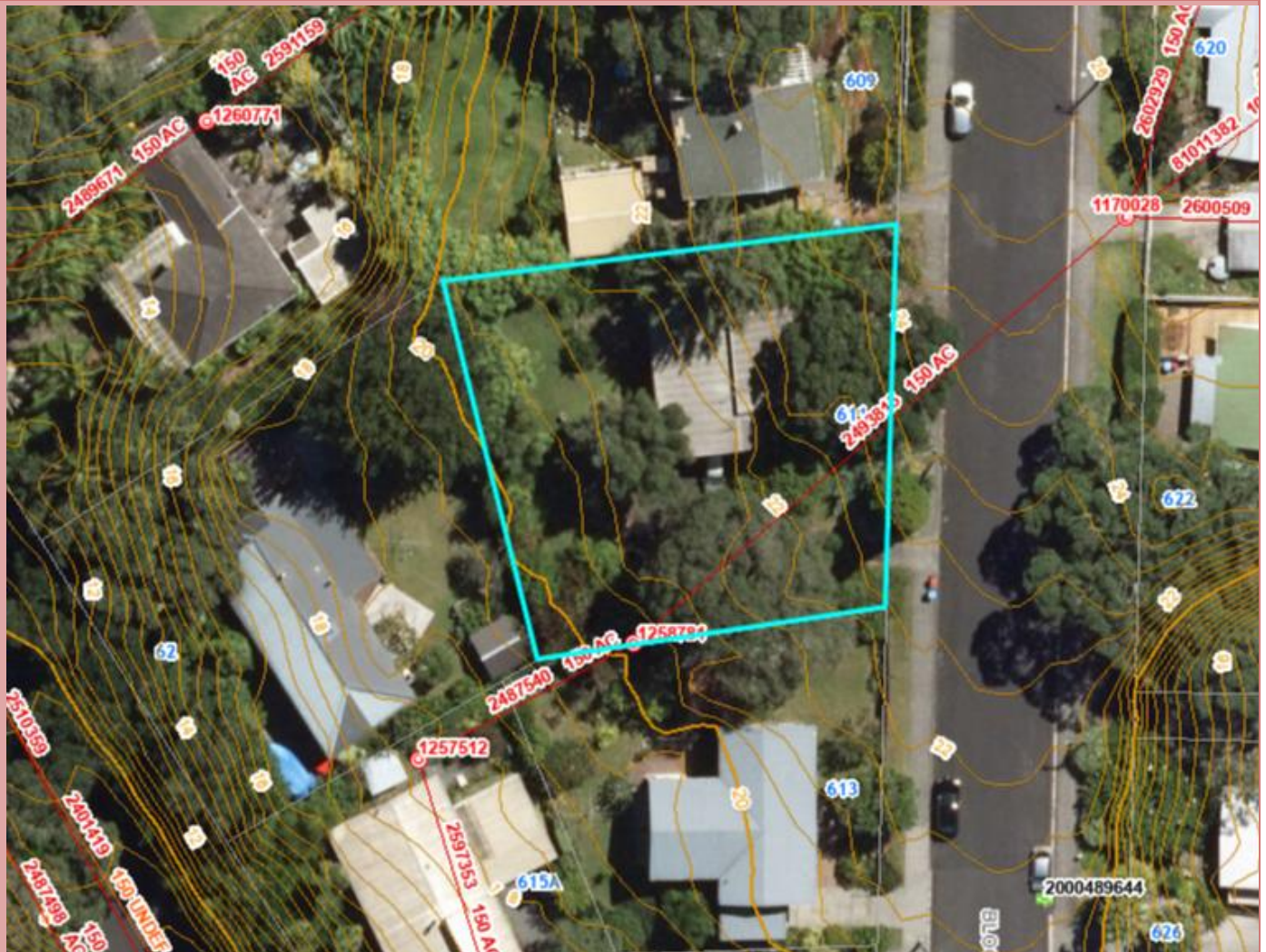
Figure 1: GIS Site aerial, showing wastewater connections (red) and stormwater (green) with contours in orange.
