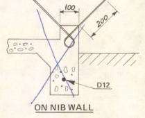
POSITION WIRE TIES AT APPROX. 1200mm CENTRES STARTING 100mm FROM CORNERS. AT ALL DOOR OPENINGS, POSITION WIRE TIES 75mm AT EACH SIDE OF DOORWAY.
