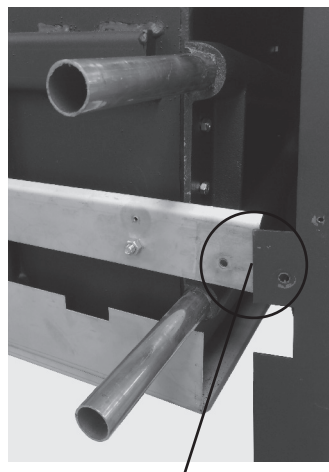
Right hand M6 bolt undone & side panel 'spread' for access
