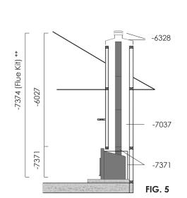
**Inbuilt Flue Installation**
