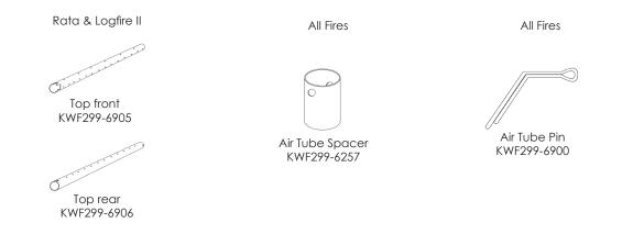
The air tube in your Kent wood fire is an important part of the appliance and helps ensure a clean, efficient and controllable burn. However, air tubes are a consumable item and need to be replaced from time to time as they are likely to degrade with continual exposure to the extreme heat generated in the fire box.
